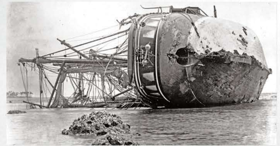
There would be no fighting between American and German ships after the hurricane. SMS Adler was photographed and beached on her side. Note the holing caused by the rocks
