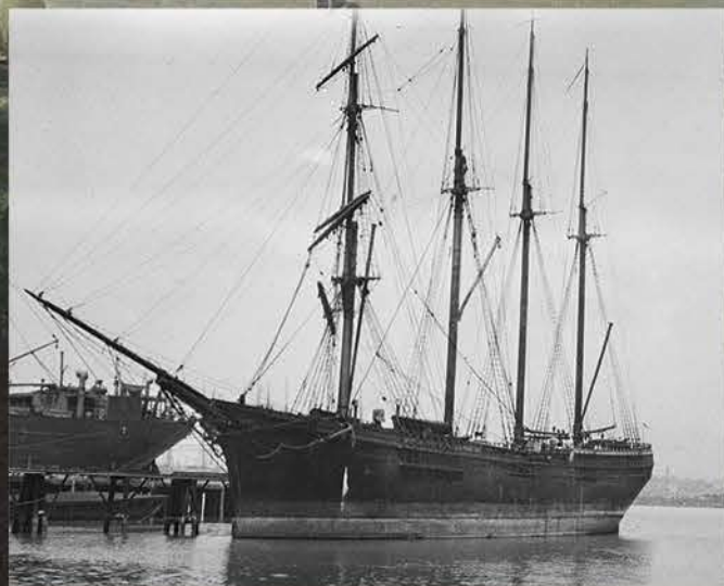
The Centennial was launched in 1875 as a three-masted Down Easter. Years later, she was rigged as a four-masted barkentine. (San Francisco Maritime National Historic Park)
