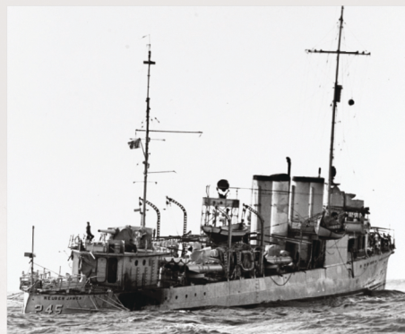
An old ship trying to keep up with the times, Reuben James mounted a 3-inch gun over the after deckhouses and twin depth charge tracks angled off the fantail. Also note towing booms port and starboard under the ship's name and the maze of rigging on fore and aft masts. The photo was taken on 30 November 1939 after the embarrassing incident when the destroyer ran aground at Lobos Cay, Cuba.
