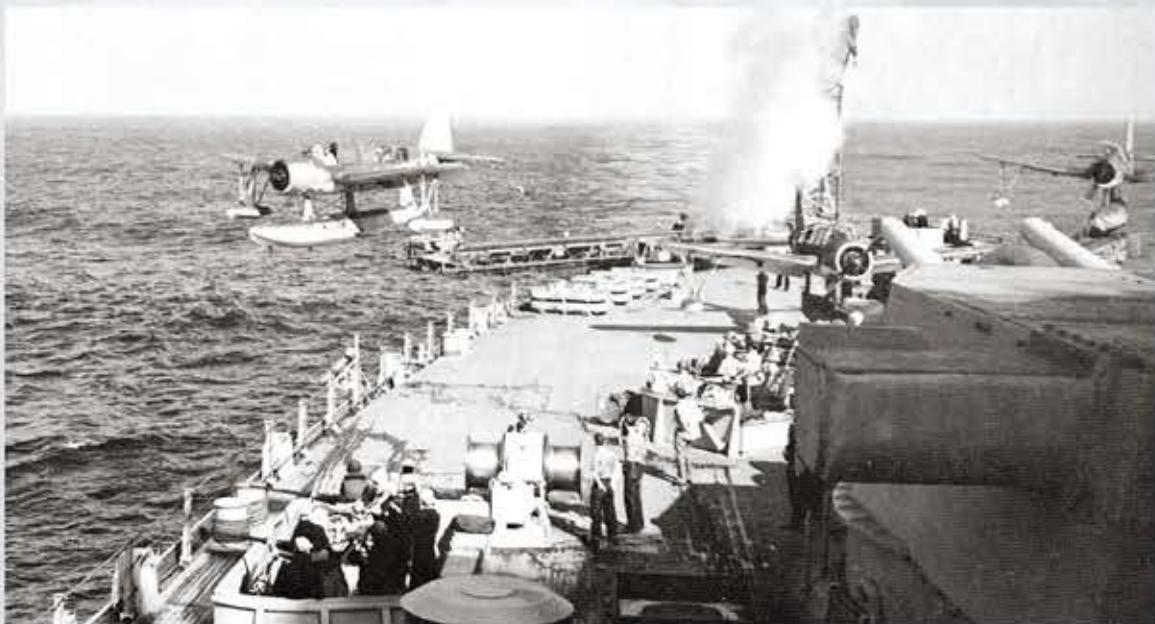
Vought OS2U-3 Kingfisher is launched off of Iowa's starboard catapult while the port catapult is prepared to launch a Kingfisher in the same direction. A third OS2U-3 is resting on a dolly on the deck. Note the many manned 20mm Oerlikon weapons. Kingfishers were ideal spotting aircraft. They could also carry depth charges and, on several occasions, they actually tangled successfully with enemy Zero fighters.
