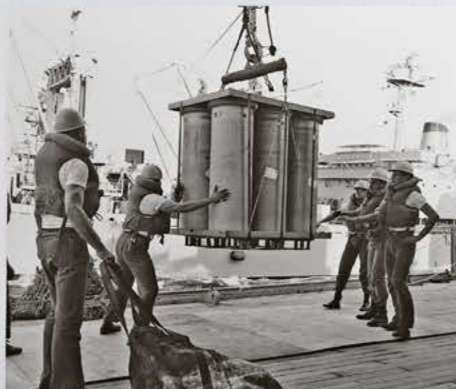
The loading and firing of the 16-inch guns was no easy task and required absolute precision from the various crews assigned to the care and feeding of the weapons. In this view, sailors receive six cans of powder for the guns. During her long and faithful service, several generations of sailors manned the big guns and this photo was taken on 4 October 1968 when the New Jersey was being replenished by the USS Haleakala (AE-25).
