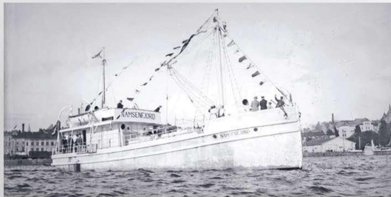
The Namsenfjord pioneered the concept of ocean-going concrete ships.
