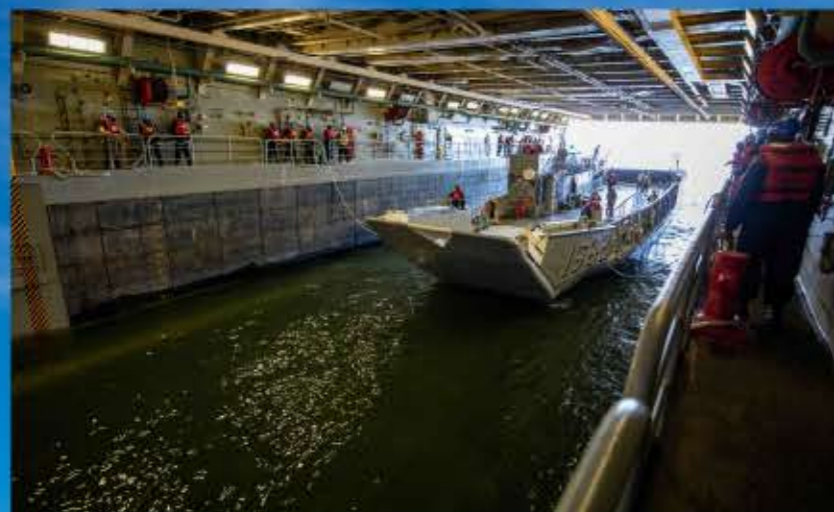
Sailors aboard the San Antonio -class amphibious transport dock ship USS Arlington (LPD-24) directs Landing Craft Utility LCU-1662 into the ship's well on 8 March 2021 in the Atlantic Ocean. (USN/John Bellino)
