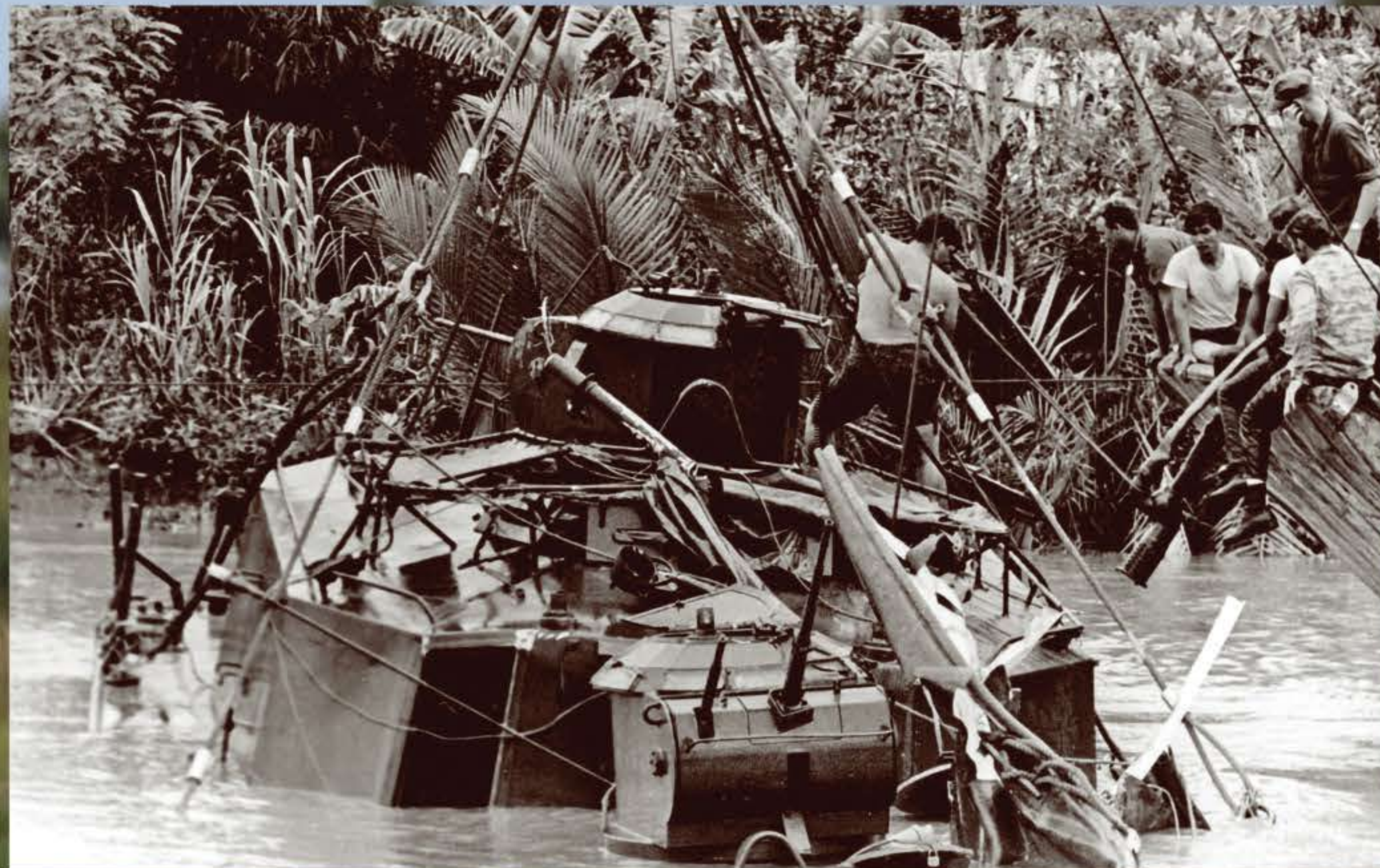
Sailors prepare a mine-damaged Assault Support Patrol Boat (ASP) for salvage.
