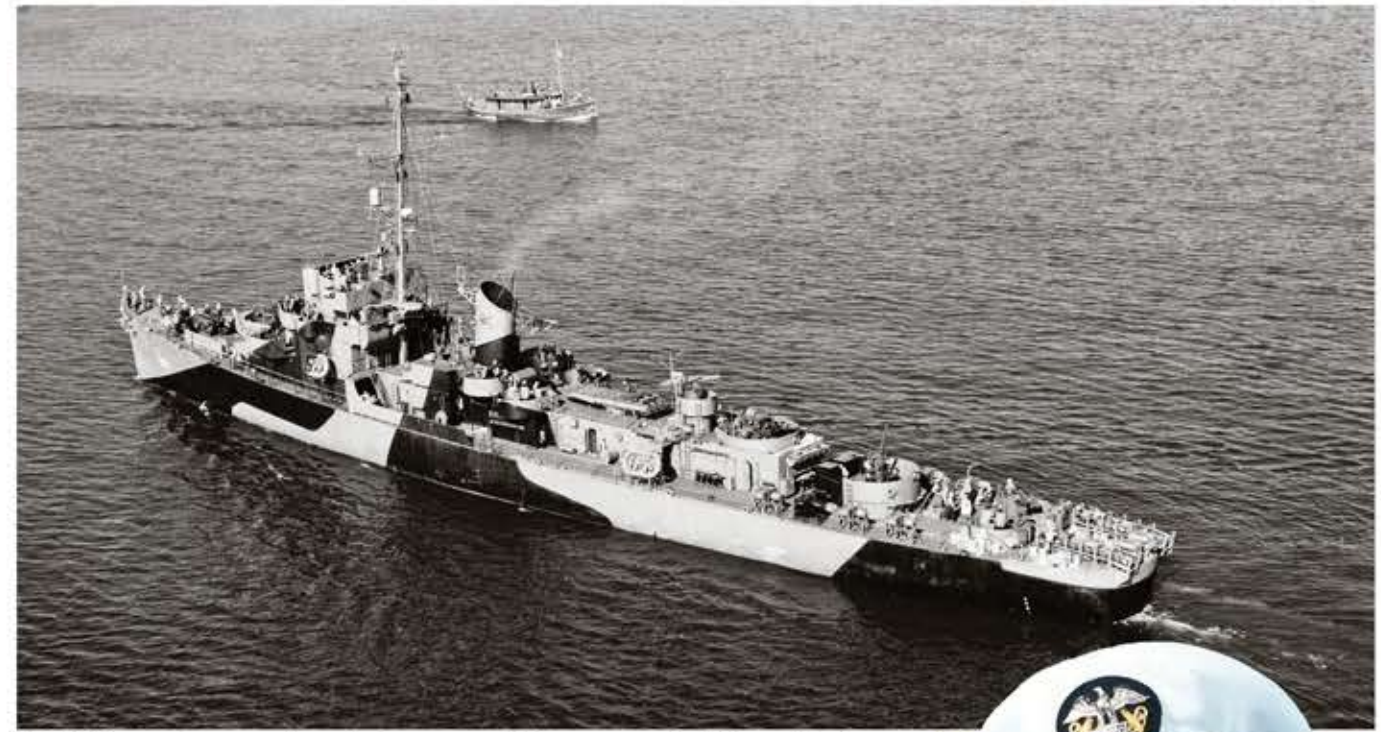
USS Tills was a Cannon -class destroyer escort. She was armed with three 3-inch Mk. 22 cannon, a twin 40mm Mk. 1 anti-aircraft mount, eight 20mm Mk. 4 anti-aircraft guns, three 21-inch torpedo tubes, one Mk. 10 Hedgehog mortar, eight Mk. 6 depth charge projectors, and two Mk. 9 depth charge tracks.
