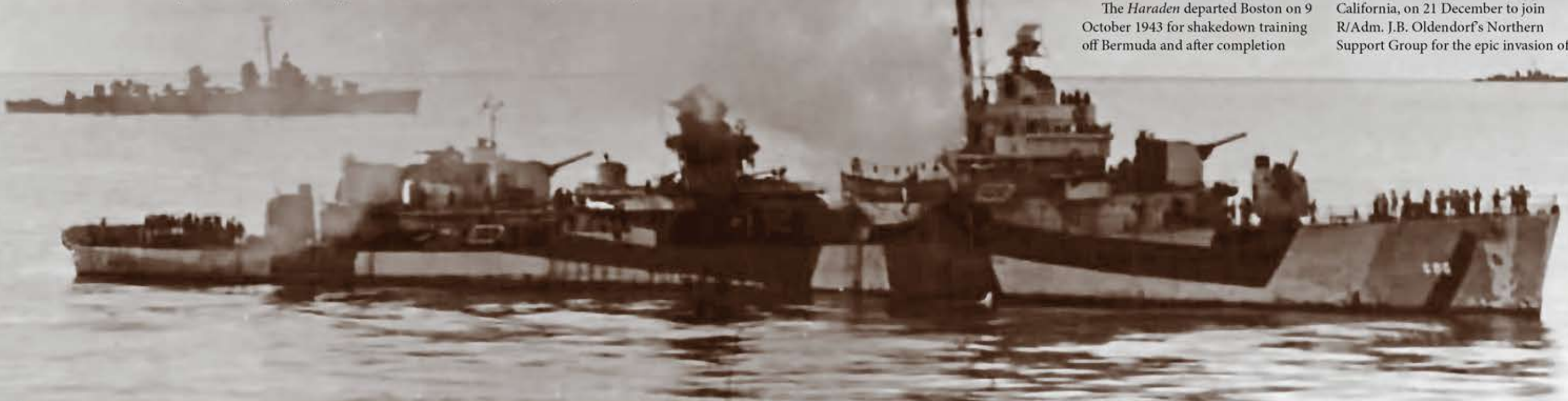
Burning after the kamikaze attack in Sulu Bay on 13 December 1944, USS Haraden is still in the water as her crew undertakes damage control. In the background, USS Twiggs is pulling in to help fight fires and offer assistance. At this point in its service life, Haraden is painted in Camouflage Measure 32, Design D.
