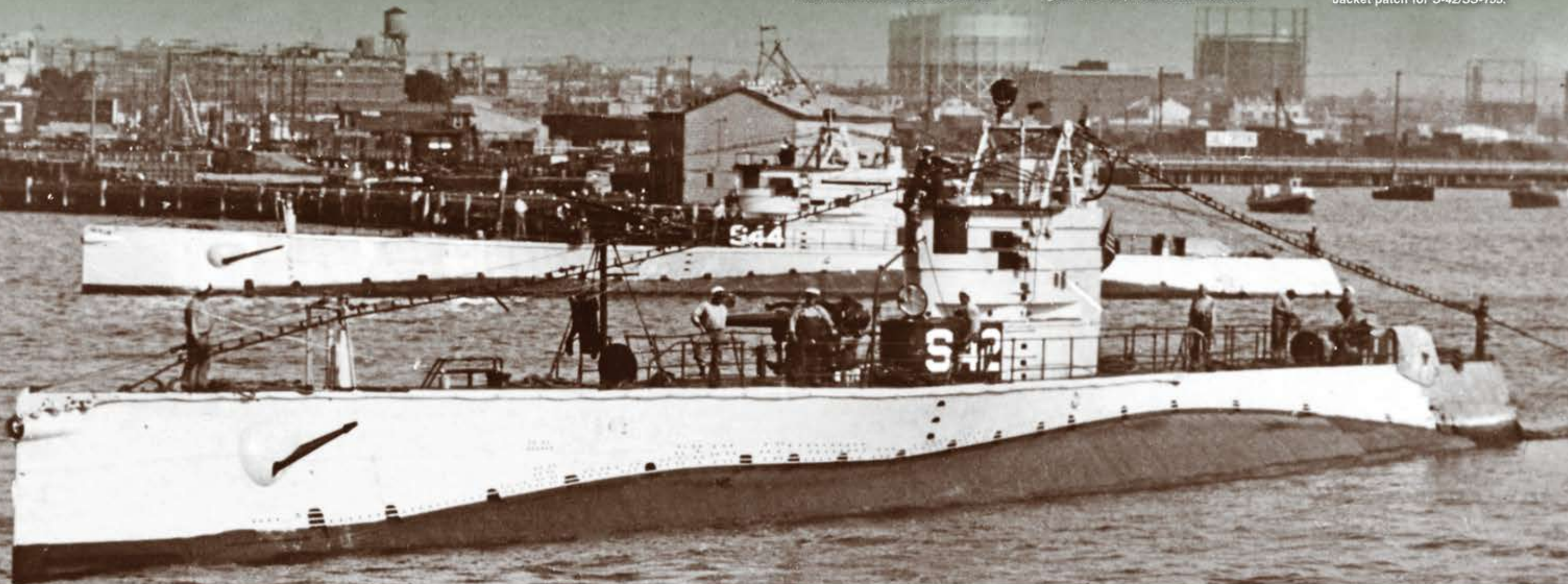
An interesting view taken during the 1930s of S-42 in the foreground with S-44 behind her. Designed during the Great War, the subs were intended for ocean operation and not coastal patrol as had earlier US Navy submarines.
